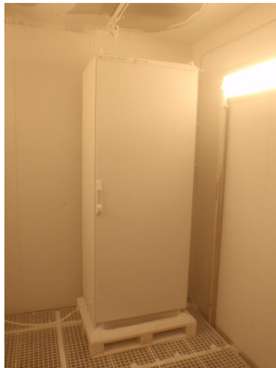
Photo 2: Inside dust chamber after IP6X test
