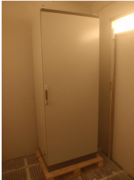
Photo 1: Inside dust chamber before IP6X test
