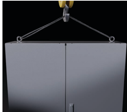
Angular bearing capacity For each eyebolt: 45 Degrees F = 2400 N 60 Degrees F = 3200 N
