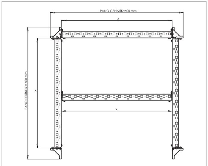
In terms of both width and interior depth size, TEOS body structure is designed at the same coefficient rate. The complete structure inside the body is designed at the 25mm coefficient. Thus, the width rail can also be installed on the depth rail.
