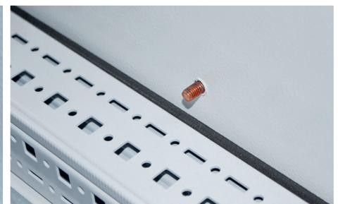
Placed on the aluminium corner combination, the earthing hooks are tightly mounted on the uncoated inner surface of the rails by means of eroding. Thereby, the earthing continuity is ensured for all rails and their parts
